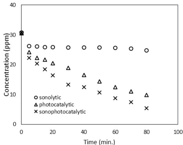
**Fig. 2** The degradation of dyestuffs at the constant parameters (at 30°C temperature, 30 % amplitude of sonolysis and 44 W/m<sup>2</sup> light intensity)
