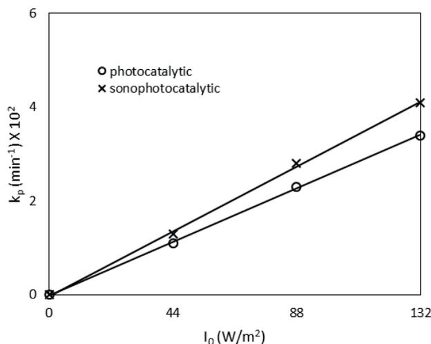
Fig. 5  $k_p$  values versus light intensities for photocatalytic and sonophotocatalytic processes
