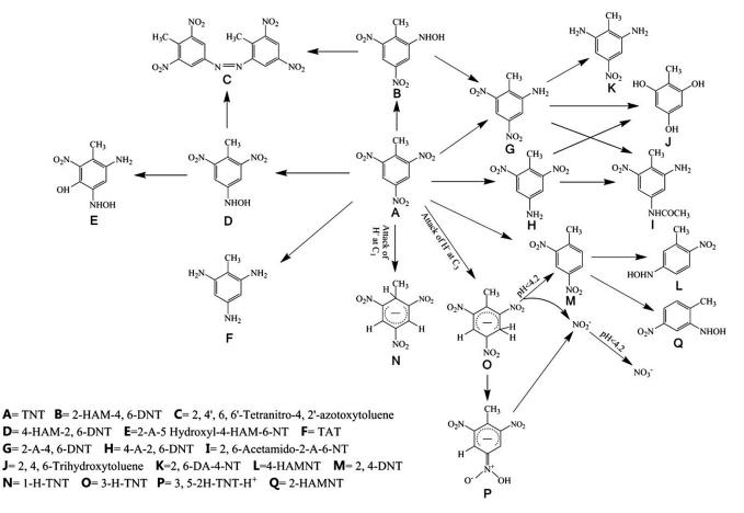
Fig. 1 Aeorbic and anaerobic TNT metabolization. It is important to note that only initial and final transformation products are represented here. 1-H-TNT, and 3, 5-2H-TNT-H<sup>+</sup>are the Meisenheimer complexes (adapted from Kalderis et al., 2011 and Ziganshin et al., 2010).
