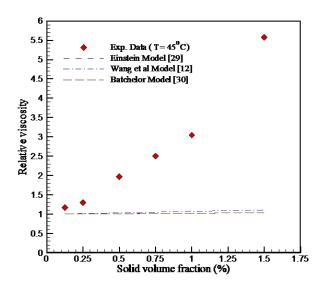
Fig. 1 The comparison between experimental data and the results obtained from theoretical models
