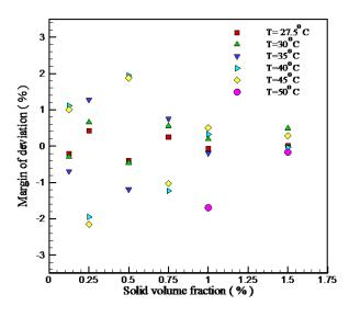
Fig. 7 Deviation of data obtained from the proposed models with experimental data
