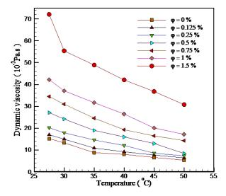
Fig. 4 Variations of viscosity in terms of temperature in different volume fractions
