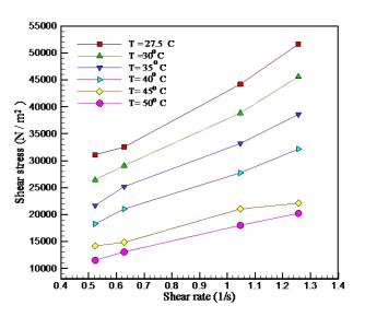
Fig. 2 Shear stress in terms of shear rate for copper oxide-water nanofluid with volume fraction of 1% in different temperatures
