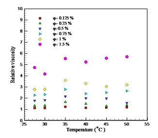
Fig. 6 Variations of relative viscosity in terms of temperature in different volume fractions
