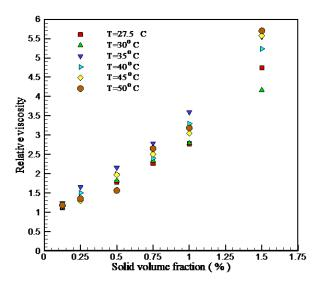
Fig. 5 Variations of relative viscosity in terms of volume fraction in different temperatures
