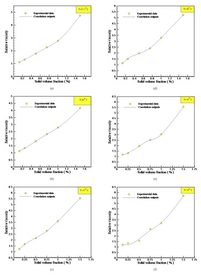
Fig. 8 A comparison between experimental data and the proposed models in (a) T = 27.5 °C (b) T = 30 °C (c) T = 35 0C (d) T = 40 °C (e) T = 45 °C (f) T = 50 °C
