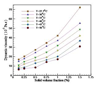
Fig. 3 Variations of viscosity in terms of volume fraction in different temperatures
