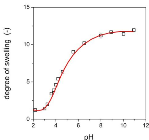
Fig. 4 Degree of swelling of PASP-10-DAB-10 hydrogel as a function of pH
