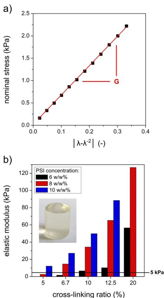
Fig. 3 a) Determination of compressive elastic modulus (sample PASP-6-DAB-10) and b) compressive elastic modulus of PASP-DAB hydrogels with different composition
