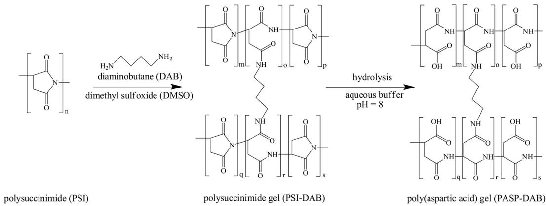
**Fig. 1** Synthesis route of poly(aspartic acid) hydrogel cross-linked with diaminobutane (PASP-DAB)
