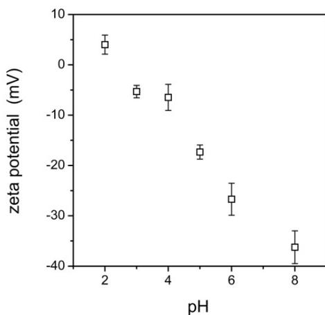
Fig. 7 Zeta potential of PASP-6-DAB-10 nanogels as a function of pH
