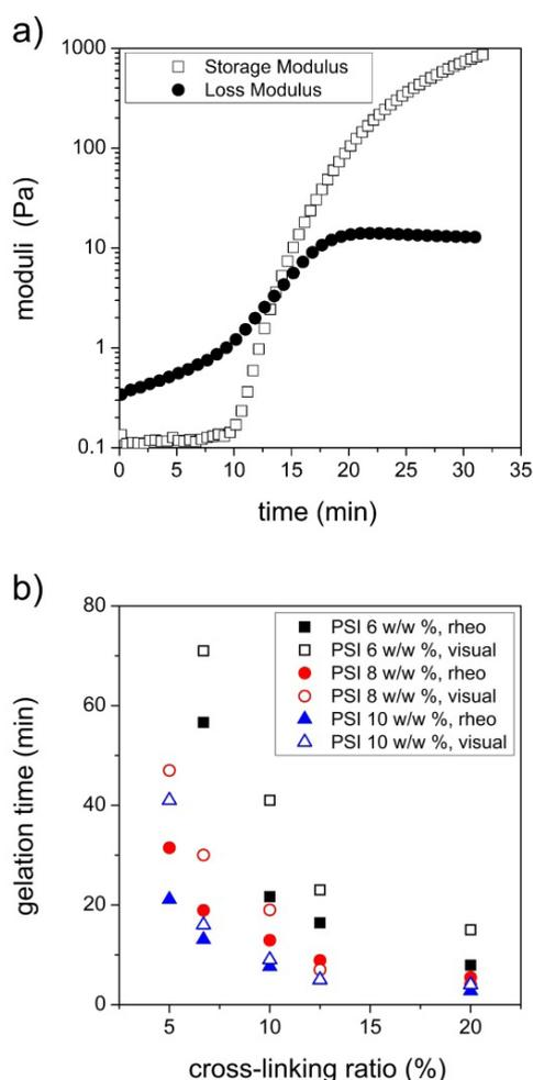
**Fig. 2** a) Simultaneous increase in the dynamic moduli around the gel point of the PSI in DMSO (PSI-6-DAB-10), gelation time was defined as the time at the equality of the two moduli and b) gelation time of PSI bulk gels cross-linked with DAB as a function of cross-linking ratio was determined by rheometry (solid symbols) and visual observation (open symbols)
