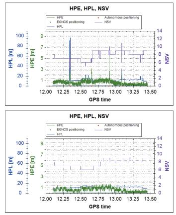
Fig. 5 The values of HPE, HPL and the number of satellites (NSV) used in "en-ruote GPS/EGNOS" mode registered during the flight (up) and on EGNOS monitoring permanent station (down)
