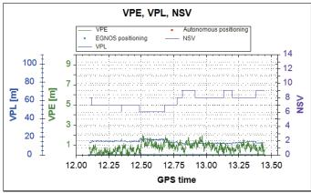
Fig. 4 The values of VPE, VPL and the number of satellites (NSV) used in "PA GPS/EGNOS" mode registered during the flight (up) and on EGNOS monitoring permanent station (down)
