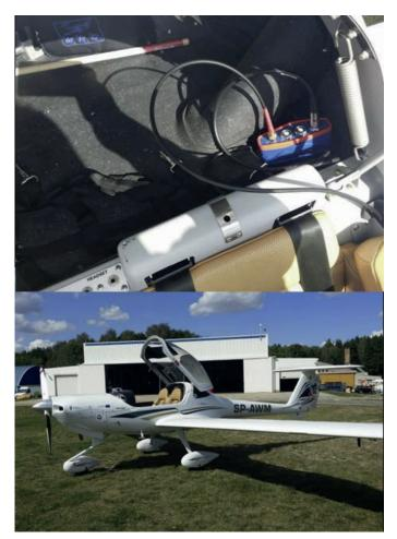
Fig. 1 The Diamond DA 20-C1 plane and measuring equipment involved in the kinematic test
