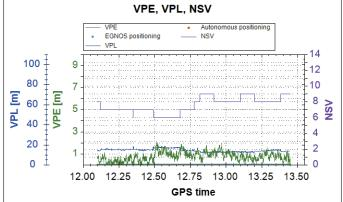
**Fig. 6** The values of VPE, VPL and the number of satellites (NSV) used in "en-ruote GPS/EGNOS" mode registered during the flight (up) and on EGNOS monitoring permanent station (down)
