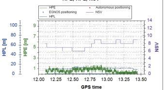
Fig. 3 The values of HPE, HPL and the number of satellites (NSV) used in "PA GPS/EGNOS" mode registered during the flight (up) and on EGNOS monitoring permanent station (down)
