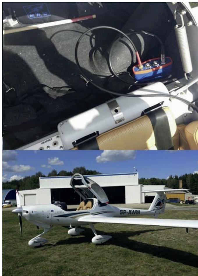
Fig. 1 The Diamond DA 20-C1 plane and measuring equipment involved in the kinematic test
