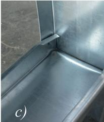
Fig 2. Failure modes of unbraced column-end elements: a) crinkling of column-end; b) mixed type; c) distortional-like failure
