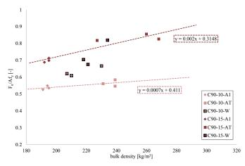
Fig. 7 Ultimate load to yield strength ratios vs. bulk density of PAC for C90
