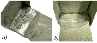
Fig. 4 Failure shapes of encased elements: a) local buckling; b) connection failure
