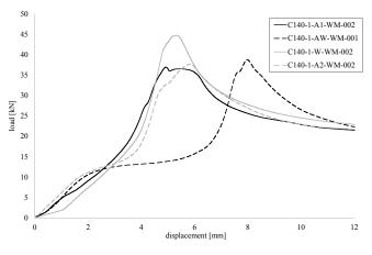
Fig. 5 Typical load-displacement curves of specimens
