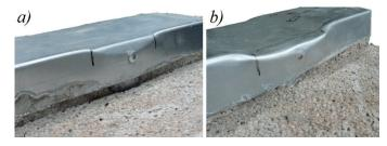
Fig. 6 Deformation of the connections: a) self-drilling screws; b) spot-welds
