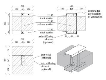
Fig. 1 Column-end joint element build-up of a C140 cross-section
