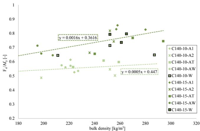
**Fig. 8** Ultimate load to yield strength ratios vs. bulk density of PAC for C140
