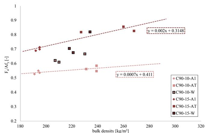
**Fig. 7** Ultimate load to yield strength ratios vs. bulk density of PAC for C90
