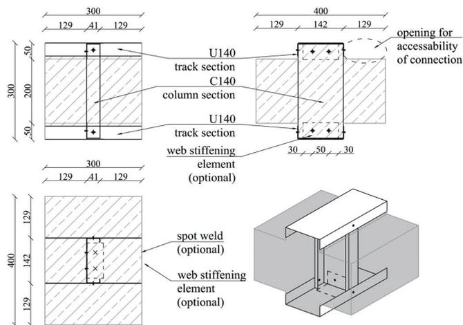
Fig. 1 Column-end joint element build-up of a C140 cross-section
