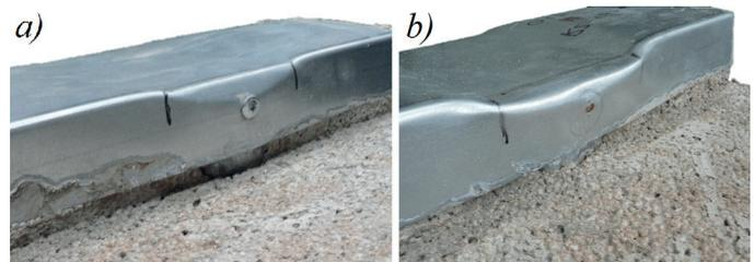
Fig. 6 Deformation of the connections: a) self-drilling screws; b) spot-welds
