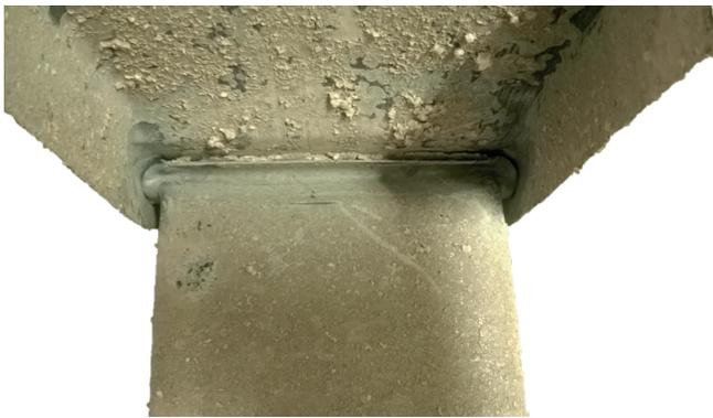
Fig. 3 Connection failure of encased elements
