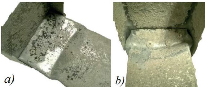
Fig. 4 Failure shapes of encased elements: a) local buckling; b) connection failure
