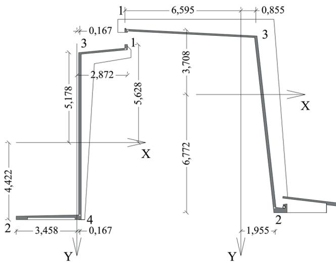
Fig. 8 Cross section of the folded plates. Position of representative points. Source: Prepared by the authors from the data provided by the original project design dossier.
