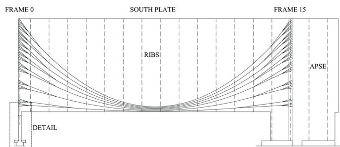
Fig. 3 Post-tensioning tendons system in South folded plate.
