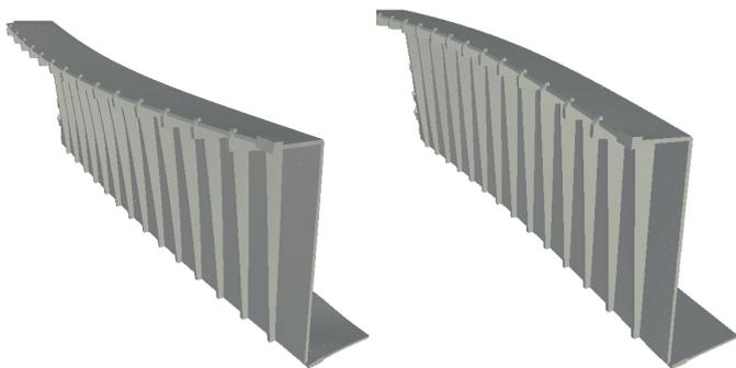
**Fig. 14** North plate. Deformations under dead loads and post-tensioning forces.
