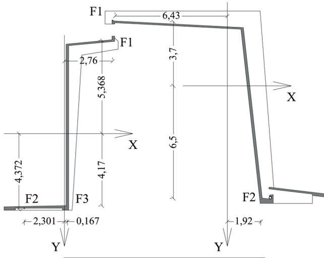
Fig. 7 Cross section of the folded plates. Loads centre and prestressing forces. Source: Prepared by the authors from the data provided by the original project design dossier.
