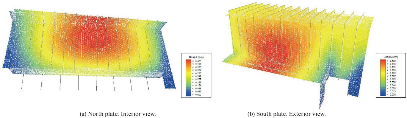
Fig. 15 Horizontal displacements caused by wind loads.
