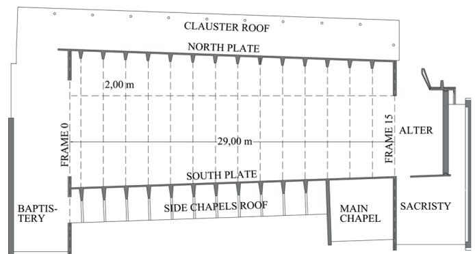
Fig. 2 Plan and structural scheme. Project of San Nicolás church (Echegaray 1959).
