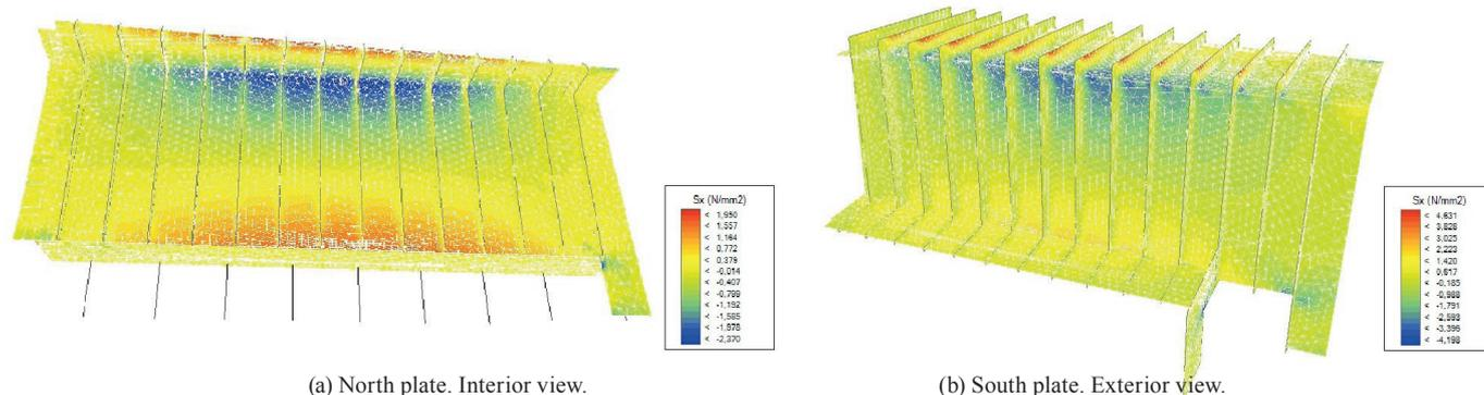
**Fig. 10** Normal stresses due by dead loads.
