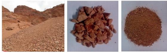
Fig. 2 The mountain, coarse and fine aggregates of spontaneous combustion gangue
