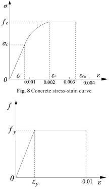
Fig. 9 Reinforcement stress-strain curve
