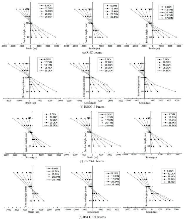
Fig. 7 The distribution curve of strain for every measuring points along the section height under the action of all levels of load
