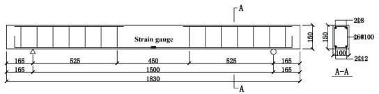
Fig. 3 Details of test beams (unit: mm)
