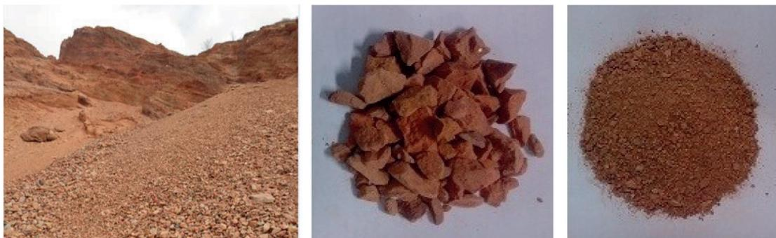
Fig. 2 The mountain, coarse and fine aggregates of spontaneous combustion gangue
