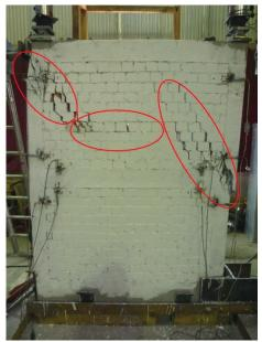
(e) Specimen Kc2 - Sp.2. - shear and bending failure
