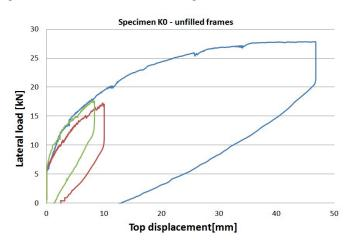
Fig. 7 Load vs. top displacement curves of unfilled test frames (two of the specimens were only loaded up to the first concrete crack, not up to collapse)
