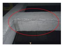
(c) Specimen K0 – Sp.1. and Sp.3. (d) Specimen K0 - Sp.1. and Sp.2. Fig. 11 Bended cracks of non-filled test frames under lateral load
