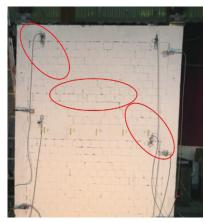
(c) Specimen Km1 - Sp.3. - corner-to-corner cracks
