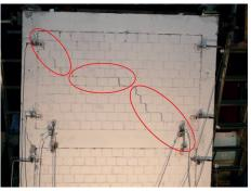
(b) Specimen Kcl - Sp.2. - corner-to corner cracks on infill
