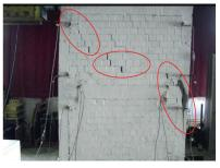
(e) Specimen Km2 - Sp.2. - failure of RC frame
