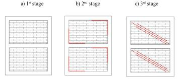
Fig. 1 Behaviour of infilled frames according to Polyakov [8]
