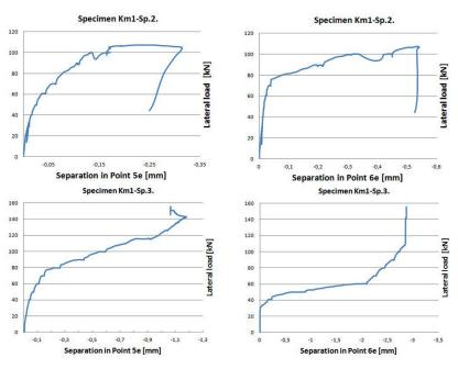
Fig. 10 Typical separation vs. load diagrams
