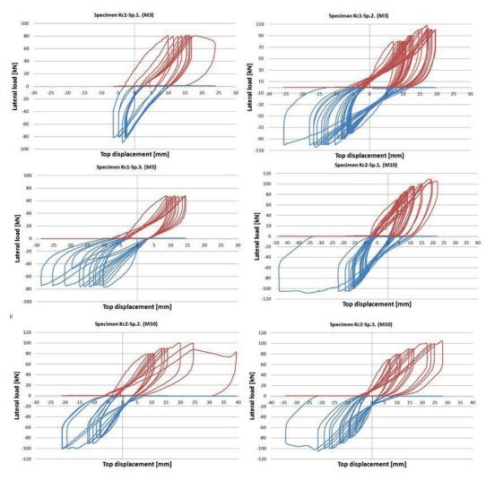
Fig. 16 Load vs. top displacement curves of the infilled test frames under cyclic load
