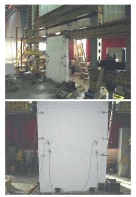
(b) The whole measurement system Fig. 13 Loading system under cyclic loading
