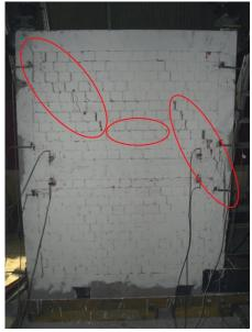
(f) Specimen Kc2 - Sp.3. - shear failure of RC frame, of RC frame, sliding along the diagonal crack diagonal cracks on infill wall
