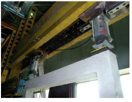
(b) Hydraulic jacks on an unfilled frame
