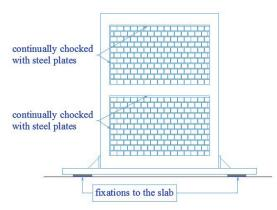
Fig. 4 The infilled frame specimen
