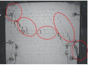
(a) Typical shear cracks on specimen
