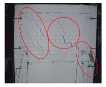
(f) Specimen Km2 - Sp.3. failure of RC frame, corner-to-corner shear cracks sliding in the middle of the wall
