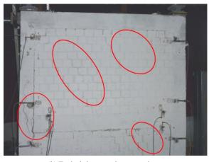
(b) Typical shear cracks on specimen Fig. 9 Typical failure modes, corner-to-corner cracks of the specimens
