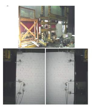
(b) The whole measurement system Fig. 14 Displacement measurements under cyclic loading
