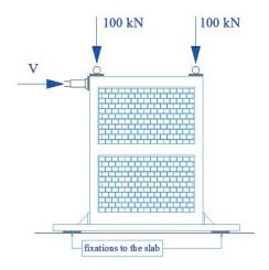
(a) Scheme of the test set-up
