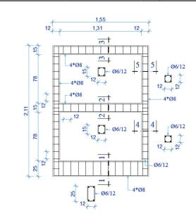
Fig. 2 Dimensions and reinforcements of the test frames
