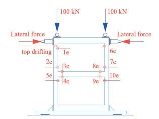
(a) Scheme of measurement points on the test frame
