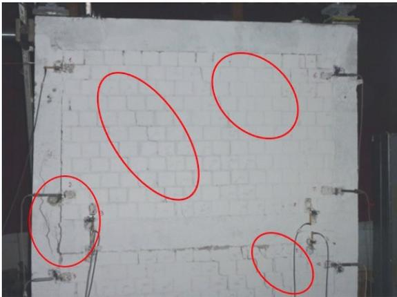
(b) Typical shear cracks on specimen
