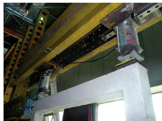
(b) Hydraulic jacks on an unfilled frame
