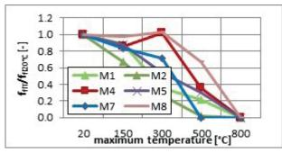
Fig. 7 Temperature-dependent relative flexural strength of reference and micro-fibre concretes (averaged from 3 measurements)
