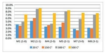
Fig. 10 Porosity values due to micro-fibres in relation to the temperature
