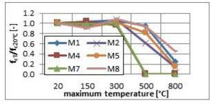
Fig. 4 Temperature-dependent relative compressive strength of reference and micro-fibre concretes (averaged from 3 measurements)
