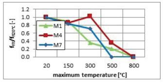
Fig. 6 Relative flexural strength values of concretes without fibres (calculated from 3 measurements) in function of temperature
