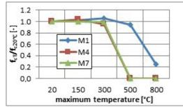
Fig. 3 Relative compressive strength values of concretes without fibres (calculated from 3 measurements) in function of temperature
