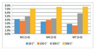
Fig. 9 Porosity values due to increased compressive strength and temperature
