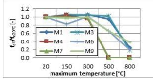
**Fig. 5** Temperature-dependent relative compressive strength of concrete with macro-fibre and without fibre (averaged from 3 measurements)
