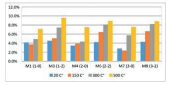
Fig. 11 Porosity values due to macro-fibres in relation to the temperature
