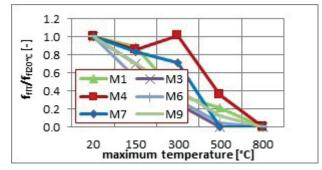
Fig. 8 Temperature-dependent relative flexural strength of concrete with macro-fibre and without fibre (averaged from 3 measurements)
