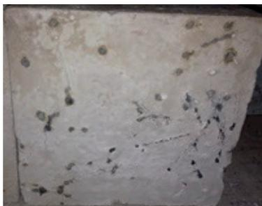
Fig. 2 The surface of macro-fibre concretes after heat loading of 300 °C
