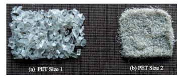
Fig. 2 PET sizes used: (a) Size 1 (2.36–1.18 mm); (b) Size 2 (300–150  $\mu m)$
