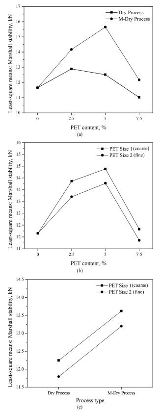
Fig. 9 Least-square mean plots for Marshall stability: (a) PET content vs. process type, (b) PET content vs. PET size, and (c) Process type vs. PET size
