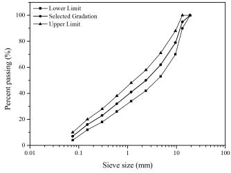
Fig. 1 Aggregate gradation curves for BC mix with specification limits
