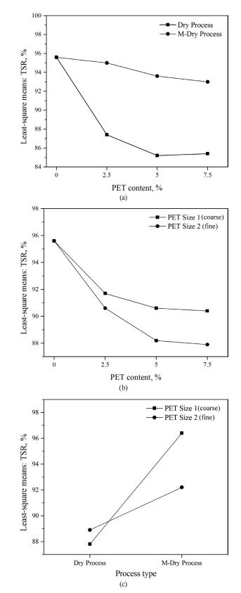
Fig. 14 Least-square mean plots for TSR: (a) PET content vs. process type, (b) PET content vs. PET size, and (c) Process type vs. PET size
