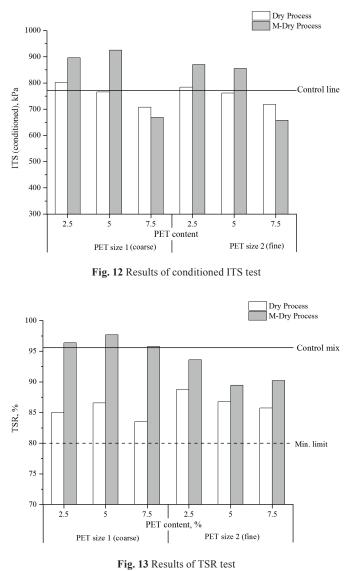
Fig. 13 shows TSR values of PET modified mixes with different PET contents, sizes and production processes. It is seen that mixes produced by modified dry process clearly outperform those with dry process in terms of resistance against moisture damage. When coarser PET size is used, the results are even better than the control mix. Nevertheless, all PET modified mixes satisfy the minimum requirement of 80% TSR.
