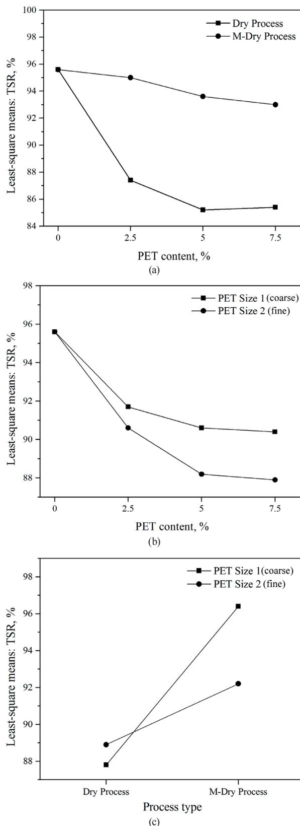
Fig. 14 Least-square mean plots for TSR: (a) PET content vs. process type, (b) PET content vs. PET size, and (c) Process type vs. PET size
