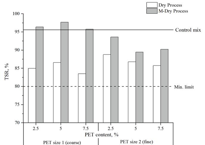
Fig. 13 Results of TSR test
