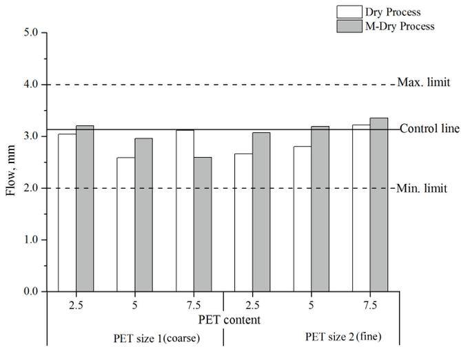
Fig. 10 Results of Marshall flow
