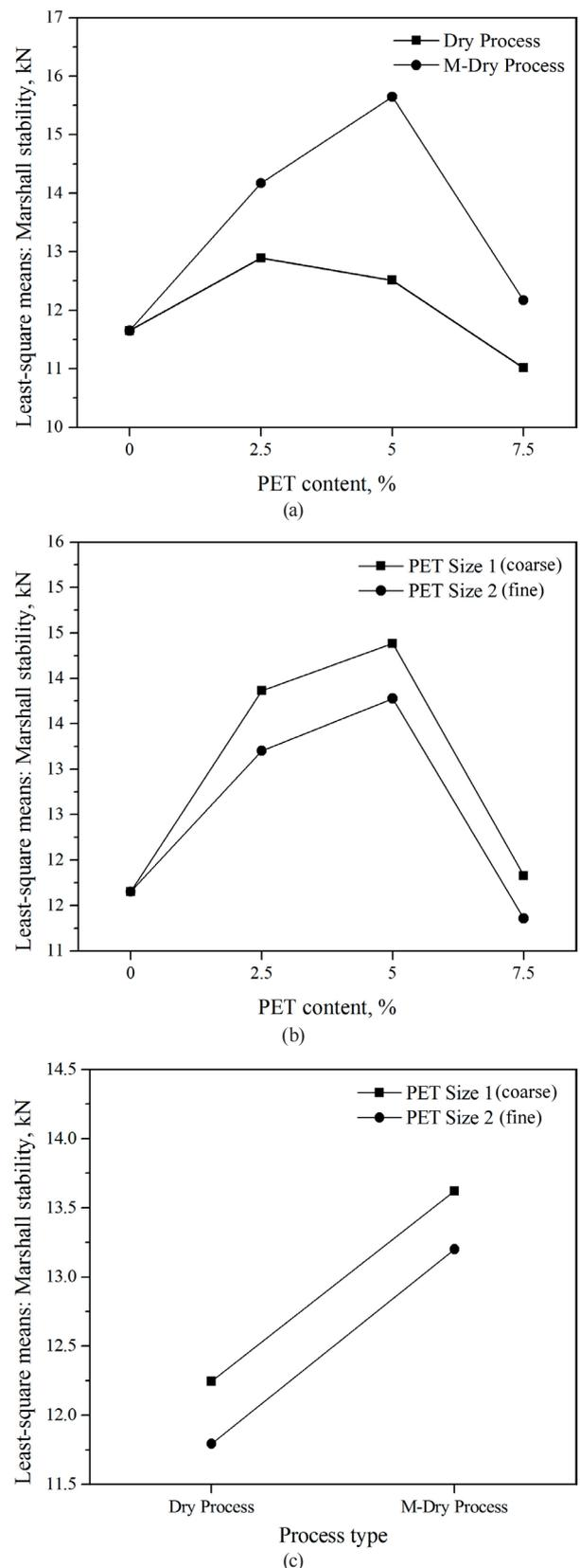
Fig. 9 Least-square mean plots for Marshall stability: (a) PET content vs. process type, (b) PET content vs. PET size, and (c) Process type vs. PET size
