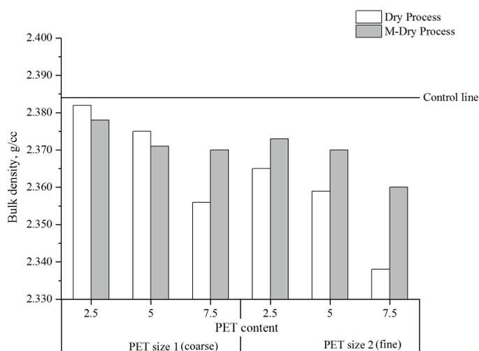
Fig. 3 Results of bulk density
