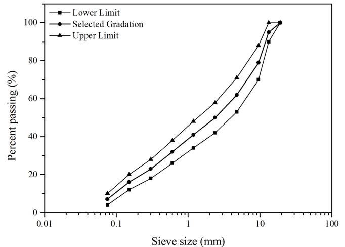
Fig. 1 Aggregate gradation curves for BC mix with specification limits
