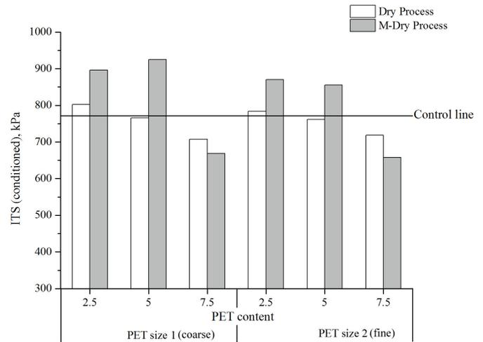
Fig. 12 Results of conditioned ITS test
