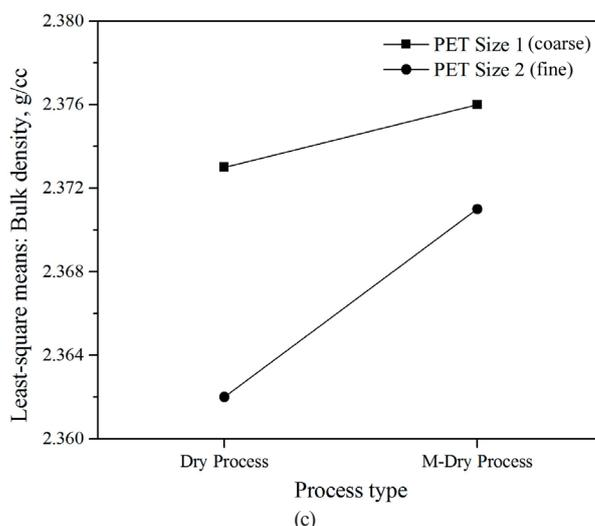
Fig. 4 Least-square mean plots for bulk density: (a) PET content vs. process type, (b) PET content vs. PET size, and (c) Process type vs. PET size
