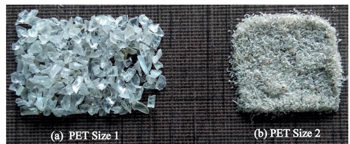
Fig. 2 PET sizes used: (a) Size 1 (2.36–1.18 mm); (b) Size 2 (300–150 µm)
