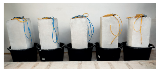
Fig. 4 Set of 5 masonry pillars with the mortars applied and probe wiring for measurement by the EIS method
