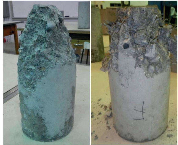
Fig. 5 Compressive failure of plain concrete (left) and fiber-reinforced concrete (right)
