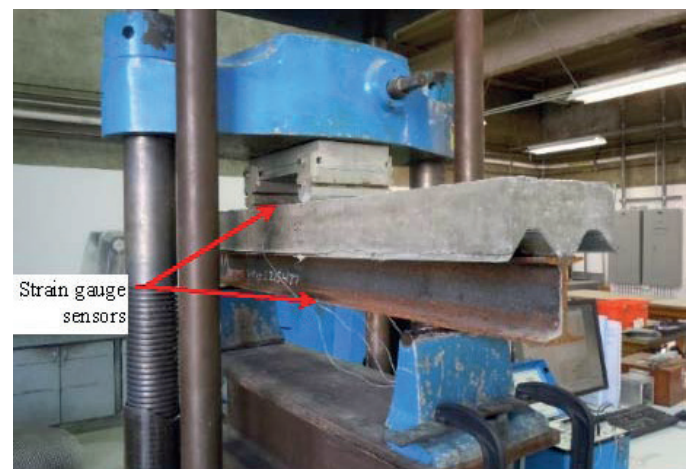
Fig. 7 Flexural test setup
