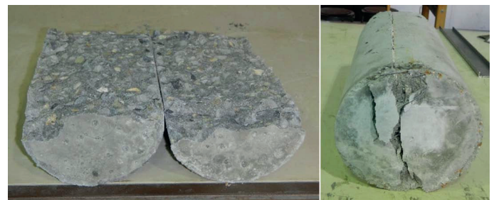
Fig. 6 Splitting tensile failure of plain concrete (left) and fiber-reinforced concrete (right)
