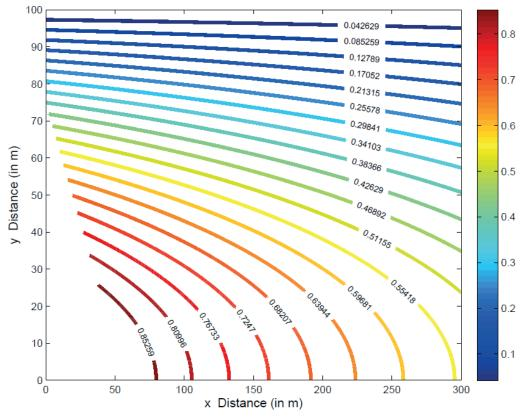
Fig. 1(b) Mode shape of the 1<sup>st</sup> natural water mode of vibration in the reservoir,  $w = w_1 = \frac{\pi c}{2H} = 22.588 \text{ rad/sec}, \ \xi = 1\%, \ T_1(x, y, w_1) = e^{-\mu x} \cos \lambda_1 y$  with  $\mu_1 = \sqrt{\lambda_1^2 - K^2}$  and  $K = \frac{w_1}{c}$ . Here c, K and  $T_1(x, y, w_1)$  are complex valued.
