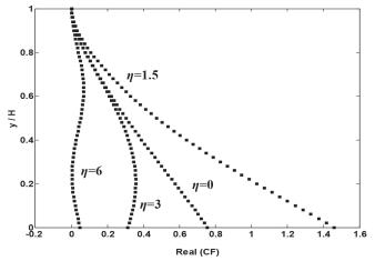
**Fig. 2** Real parts of total shear forces on a rigid dam with sloping angle  $\theta$  = 37.6° and C = 0.75 (undamped fluid case,  $\xi$  = 0%)
