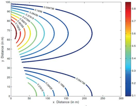
Fig. 2(b) Mode shape of the 2<sup>nd</sup> natural water mode of vibration in the reservoir,  $w = w_2 = \frac{3\pi c}{2H} = 67.76 \text{ rad/sec}$ ,  $\xi = 1\%$ ,  $T_2(x, y, w_2) = e^{-\mu_x} \cos \lambda_2 y$  with  $\mu_2 = \sqrt{\lambda_2^2 - K^2}$  and  $K = \frac{w_2}{c}$ . Here c, K and  $T_2(x, y, w_2)$  are complex valued.
