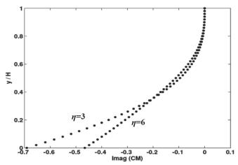
Fig. 5 Imaginary parts of total overturning moments on a rigid dam with sloping angle  $\theta = 37.6^{\circ}$  and C = 0.75 (undamped fluid case,  $\xi = 0\%$ )
