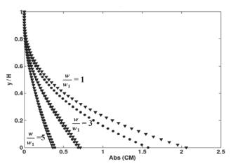
Fig. 9 Distribution of total overturning moments on a partially inclined dam with sloping angle  $\theta = 37.6^{\circ}$  and C = 0.75, for damping ratios  $\xi = 1\%$  (Triangle marker) and  $\xi = 5\%$  (Circle marker)
