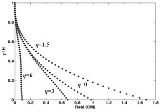
Fig. 4 Real parts of total overturning moments on a rigid dam with sloping angle  $\theta = 37.6^{\circ}$  and C = 0.75 (undamped fluid case,  $\xi = 0\%$ )
