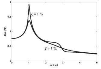
**Fig. 7** Total shear forces on a partially inclined dam with sloping angle  $\theta$  = 37.6° and C = 0.75, for damping ratios  $\xi$  = 1% and  $\xi$  = 5%
