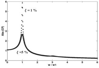
Fig. 6 Total shear forces on a rigid dam with a vertical upstream face for damping ratios  $\zeta = 1\%$  and  $\zeta = 5\%$
