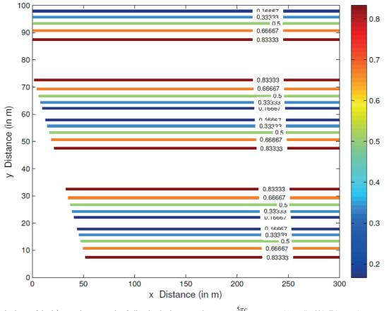
Fig. 3(a) Mode shape of the 3<sup>rd</sup> natural water mode of vibration in the reservoir,  $w = w_3 = \frac{5\pi c}{2H} = 112.94 \text{ rad} / \sec, \xi = 0\%, T_3(x, y, w_3) = e^{-\mu_x} \cos\lambda_3 y$  with  $\mu_3 = \sqrt{\lambda_3^2 - K^2}$  and  $K = \frac{w_3}{c}$ .
