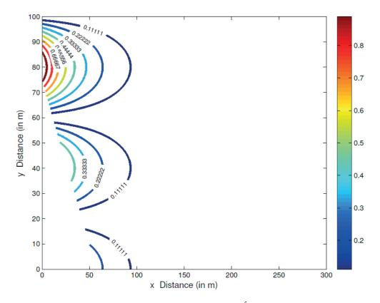
Fig. 3(b) Mode shape of the 3<sup>rd</sup> natural water mode of vibration in the reservoir,  $w = w_3 = \frac{5\pi c}{2H} = 112.94 \text{ rad / sec}$ ,  $\xi = 1\%$ ,  $T_3(x, y, w_3) = e^{-\mu x} \cos \lambda_3 y$  with  $\mu_3 = \sqrt{\lambda_3^2 - K^2}$  and  $K = \frac{w_3}{c}$ . Here c, K and  $T_3(x, y, w_3)$  are complex valued.
