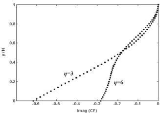
Fig. 3 Imaginary parts of total shear forces on a rigid dam with sloping angle  $\theta = 37.6^{\circ}$  and C = 0.75 (undamped fluid case,  $\xi = 0\%$ )
