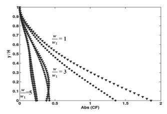
Fig. 8 Distribution of total shear force on a partially inclined dam with sloping angle  $\theta = 37.6^{\circ}$  and C = 0.75, for damping ratios  $\zeta = 1\%$  (Triangle marker) and  $\zeta = 5\%$  (Circle marker)
