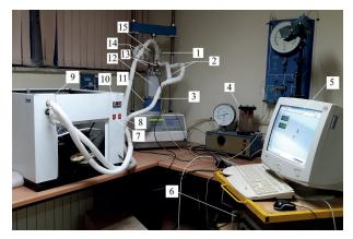
Fig. 2 Triaxial compression apparatus for frozen soils: (1) LVDT, (2) coolant output, (3) confining pressure valve, (4) confining pressure system, (5) computer system, (6) data acquisition, (7) pump power, (8) cooling power, (9) cooling machine, (10) thermostat-thermometer, (11) deviator stress system, (12) triaxial chamber, (13) thermal transducer, (14) coolant input, (15) load cell.General layout of a freeze pipe
