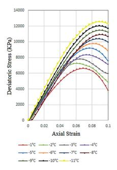
Fig. 8 Stress-strain behavior of frozen SP soil at different temperatures at confining pressure of 200 kPa and strain rate of 1 mm/min.
