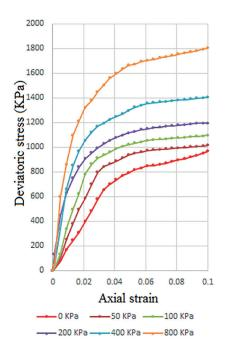
Fig. 11 Effect of confining pressure on stress-strain behavior of the frozen CL soil at temperature –3°C and strain rate 1 mm/min.
