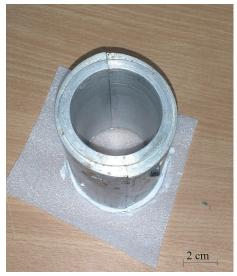
Fig. 6 Aluminium sleeve curing mold
