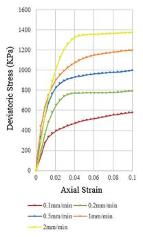
Fig. 9 Effect of strain rate on stress-strain behavior of the frozen CL soil at confining pressure 200 kPa and temperature  $-3^{\circ}C$ .
