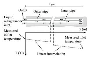
Fig. 1 General layout of a freeze pipe (after Pimentel et al.) [16]
