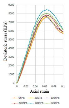
Fig. 12 Effect of confining pressure on stress-strain behavior of the frozen SP soil at temperature –3°C and strain rate 1 mm/min.
