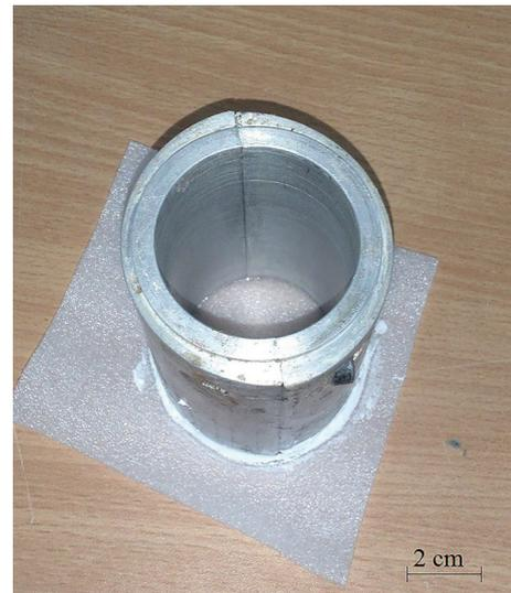
Fig. 6 Aluminium sleeve curing mold
