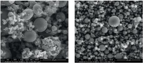
c) Siliceous Fly Ash of category N d) Siliceous Fly Ash of category S Fig. 1 Morphology of calcareous and siliceous fly ash
