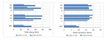
**Fig. 6** Influence of CFA with separated fractions over 0,09 mm (DS) and over 0,063 mm (CS) on rheological properties of mortars from cement G
