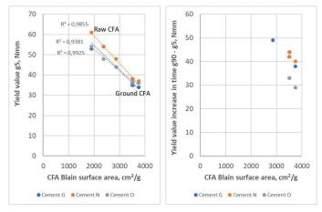
Fig. 9 CFA Blaine surface area vs yield value g and increase of yield value g in time of mortars (20% CFA type A).
