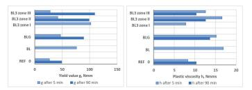
Fig. 7 Influence of CFA from selective collection on rheological properties of mortars from cement G
