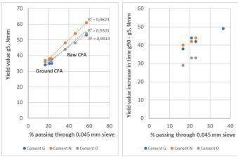
Fig. 8 CFA fineness vs yield value g and increase of yield value g in time of mortars (20% CFA type A).
