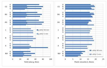
Fig. 4 Influence of CFA processing by grinding on rheological properties of mortars from cement G, N, O
