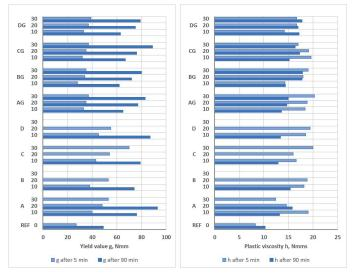
Fig. 3 Influence of the amount of CFA and its processing by grinding on rheological properties of mortars from cement G
