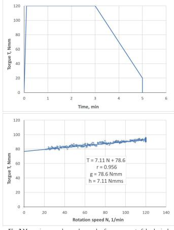
Fig. 2 Measuring procedure and example of measurement of rheological properties of mortars
