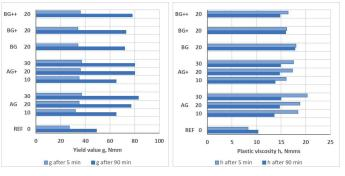
Fig. 5 Influence of the content and fineness rate of CFA on rheological properties of mortars from cement G
