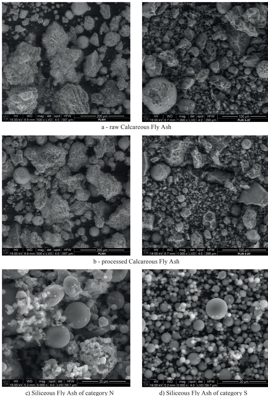
**Fig. 1** Morphology of calcareous and siliceous fly ash
