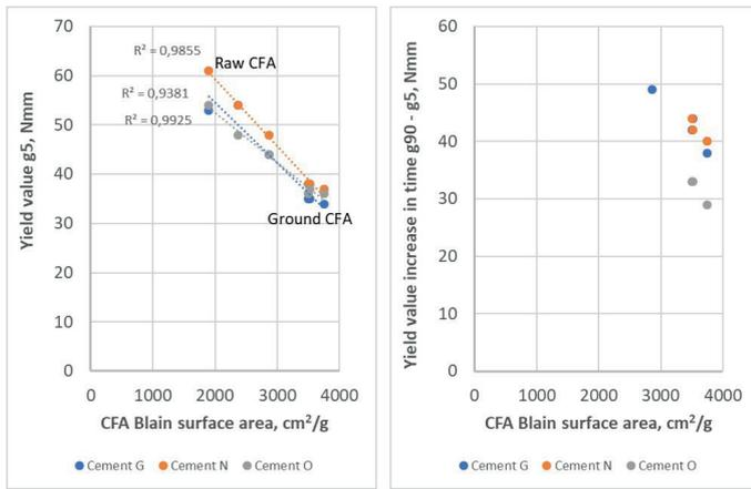
Fig. 9 CFA Blaine surface area vs yield value  $g$  and increase of yield value  $g$  in time of mortars (20% CFA type A).
