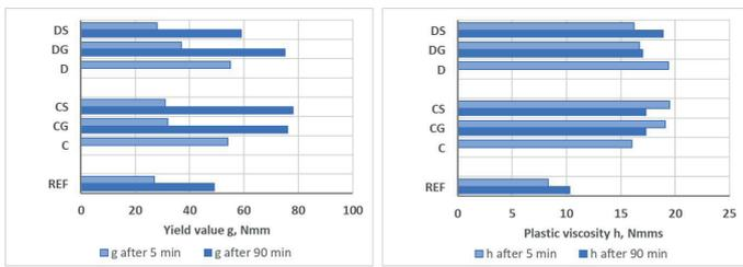
Fig. 6 Influence of CFA with separated fractions over 0,09 mm (DS) and over 0,063 mm (CS) on rheological properties of mortars from cement G
