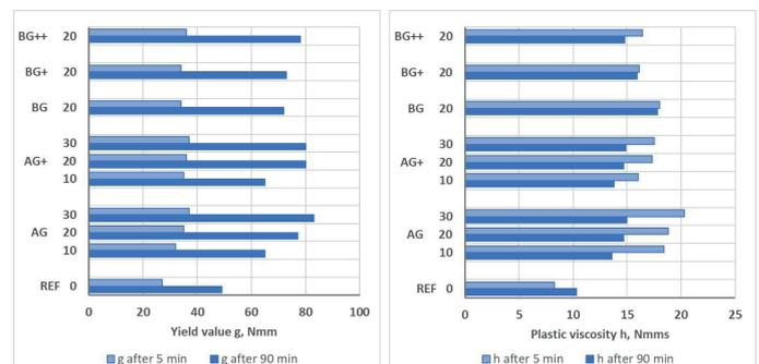
**Fig. 5** Influence of the content and fineness rate of CFA on rheological properties of mortars from cement G
