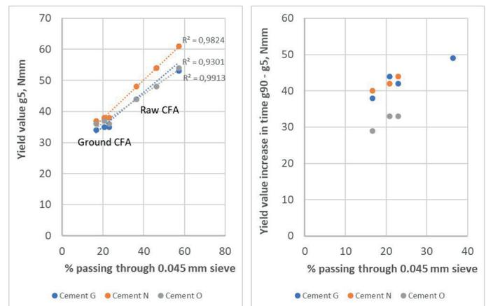
Fig. 8 CFA fineness vs yield value  $g$  and increase of yield value  $g$  in time of mortars (20% CFA type A).
