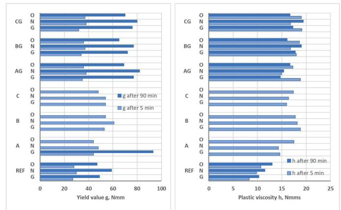
**Fig. 4** Influence of CFA processing by grinding on rheological properties of mortars from cement G, N, O
