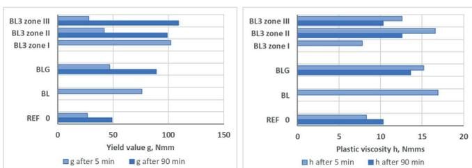
Fig. 7 Influence of CFA from selective collection on rheological properties of mortars from cement G
