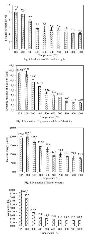
Fig. 7 Gradual weight loss determined using thermogravimetry
