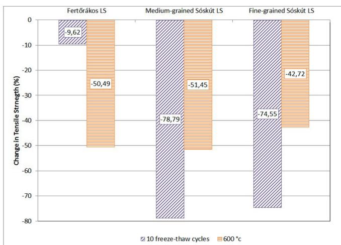
Fig. 8 Change in tensile strength after 10 freeze-thaw cycles and heating up to 600 °C
