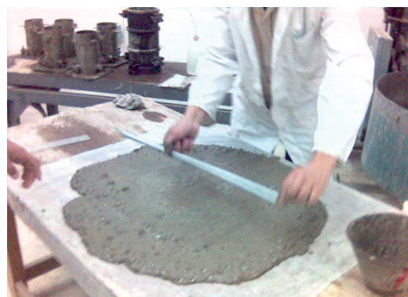
Fig. 8 Slump flow test by Abrams cone
