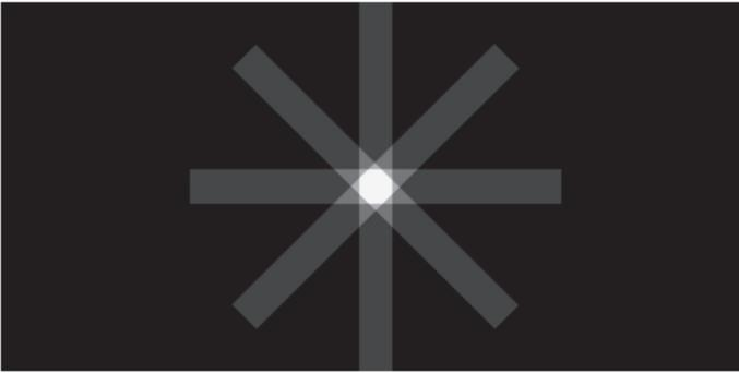
Fig. 3 Reconstructed object with the star artefact.
