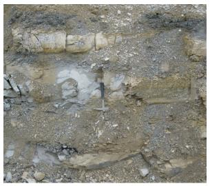
Fig. 3 Disintegration of marlstone in to different grain size in the nature
