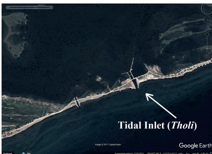
**Fig. 2** Existing formation of tidal inlets with jetties (upper) Eastern Kleisova, (lower) Tholi, as seen from Google Earth [9]
