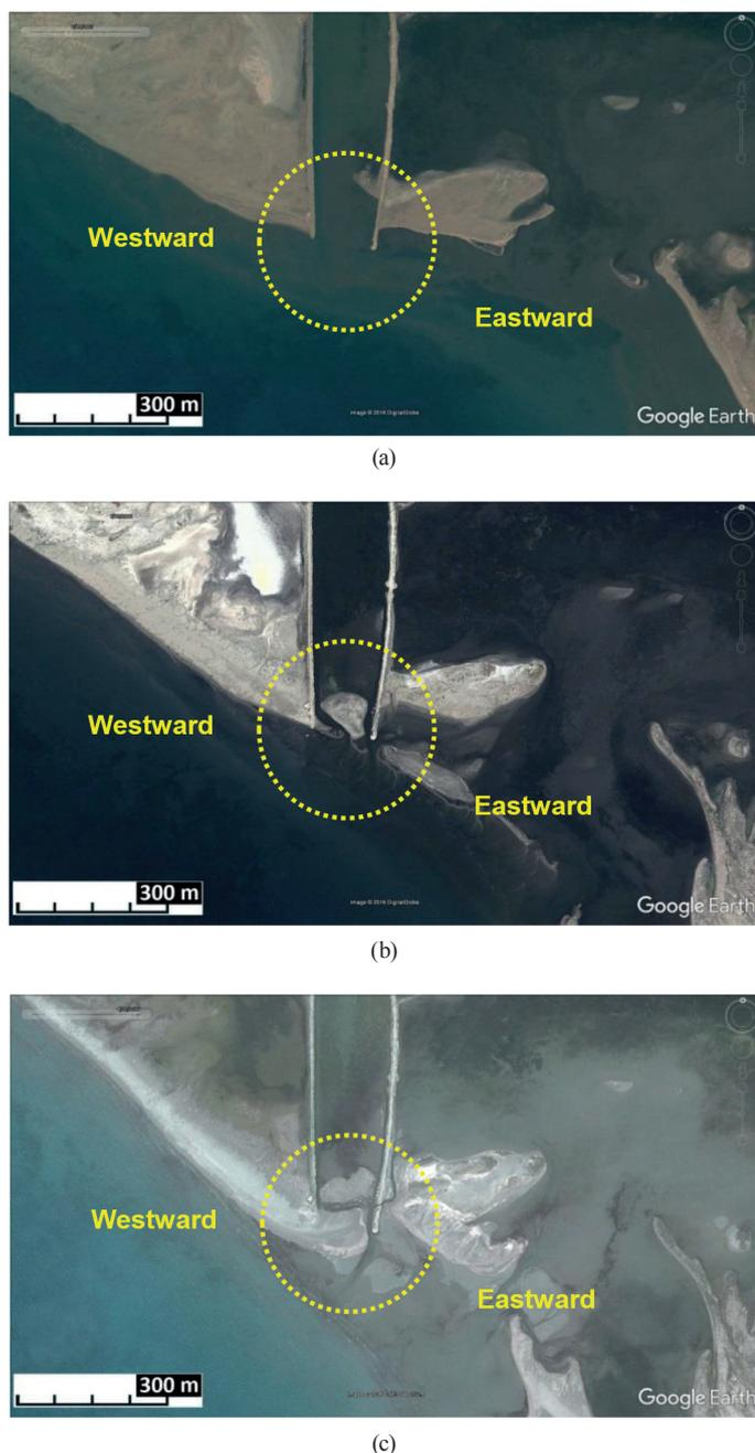
**Fig. 8** The sequence of events leading to the formation of the sandy islet in front and inside the tidal inlet, for the case of Eastern Kleisova. Satellite images from Google Earth, (a) 2007, (b) 2012, (c) 2016 [9].
