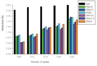
Fig. 11 Mass losses of lightweight concretes up to the 90<sup>th</sup> cycles due to  $Na_sSO_4$
