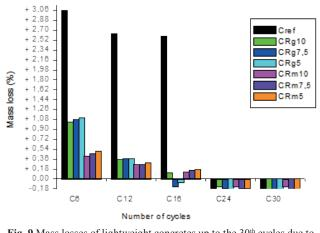
Fig. 9 Mass losses of lightweight concretes up to the 30<sup>th</sup> cycles due to  $Na_2SO_4$
