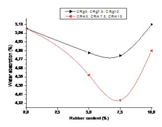
Fig. 2 Evolution of water absorption of lightweight concretes
