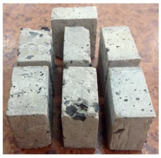
Fig. 5 Specimens of lightweight concretes after 100 freeze-thaw cycles
