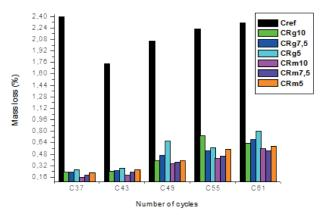
Fig. 10 Mass losses of lightweight concretes up to the 60<sup>th</sup> cycles due to  $Na_2SO_4$
