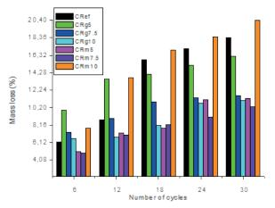
Fig. 13 Mass losses of lightweight concretes up to the  $30^{th}$  cycles of HCl attack
