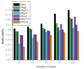
Fig. 4 Mass losses of lightweight concretes due to freeze-thaw up to the 100<sup>th</sup> cycle
