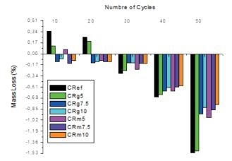
Fig. 3 Mass losses of lightweight concretes due to freeze-thaw up to the  $50^{\rm th}$  cycle
