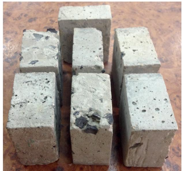
Fig. 5 Specimens of lightweight concretes after 100 freeze-thaw cycles
