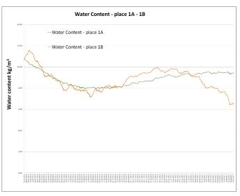
Fig. 10 Simulation results involving the changes of water content over the time of 1 year, in the vicinity of imperfections in the form of insulation connectors (A1 and A2)
