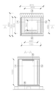
Fig. 1 Research model of the two-layer wall
