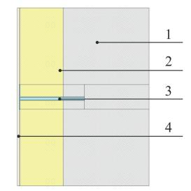
1 – wall from cellular concrete blocks, 2 – thermal insulation, 3 – connector for thermal insulation, 4 – thin-coat external plaster, adhesive with a mesh as in the ETICS system.
