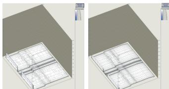
Fig. 7 Calculation results from the program WUFI 2-D. Variant 1 – external plaster  $\mu = 10$ . Envelope model as in Fig.4 in 3D view. Fig. on the left – model after 0h. Fig. on the right – model after 8760h (1 year)
