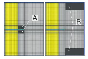
Fig. 5 A FEM mesh. The investigated area in terms of moisture increment at the edge of the model (place B) and the place of insulation connector (place A) – marked with black colour
