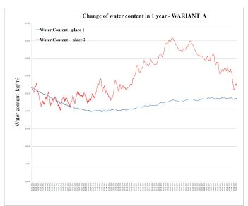
Fig. 6 Change of water content within the area of structural material around the connector and away from the connector over the time of 1 year. Variant 1
