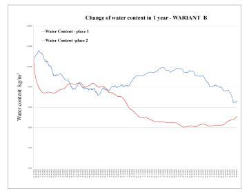
Fig. 8 Change of water content within the area of structural material around the connector and away from the connector over the time of 1 year. Variant 2
