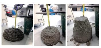
Fig. 4 Illustration of slump testing: sample 3-RCA<sub>FA</sub> in 0, 45 and 90 minute, from left to right
