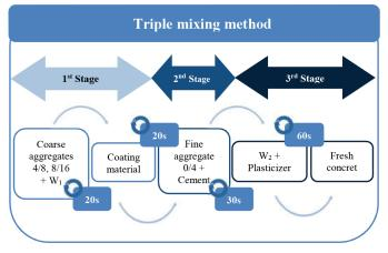
Fig. 3 Scheme of mixing course used in the experiment
