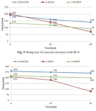
Fig. 6 Slump loss of concrete mixtures with NA
