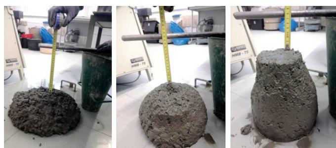
**Fig. 4** Illustration of slump testing: sample 3-RCA<sub>FA</sub> in 0, 45 and 90 minute, from left to right
