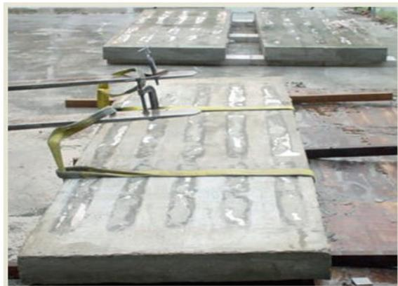
Fig. 5 AAC-concrete lightweight precast ferrocement composite floor slab
