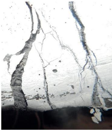
Fig. 15 Fiber bridging effects in ECC layer
