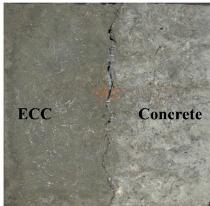
Fig. 12 Surface interface failure under split load
