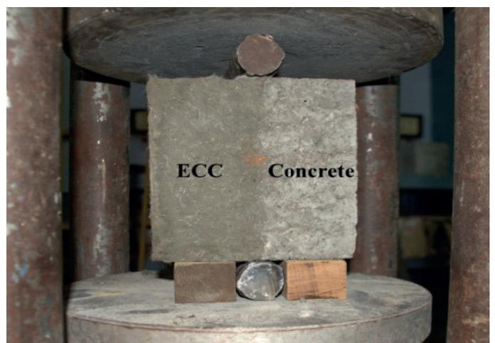
**Fig. 3** Bond test on conventional concrete cube
