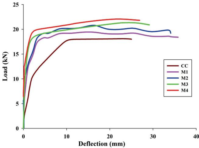
Fig. 14 Load Deflection curve of various beam
