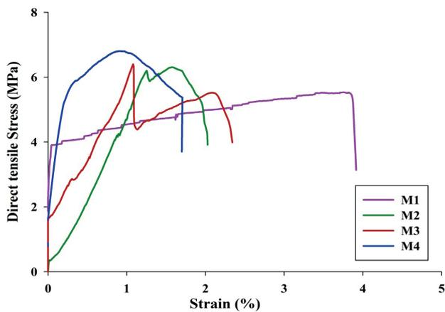
Fig. 9 Stress strain curve of direct tensile test
