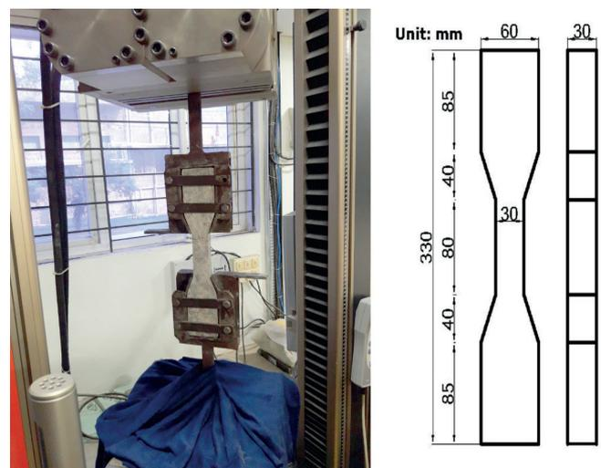
**Fig. 2** Direct tensile test specimen detail (Dog Bone Specimen)
