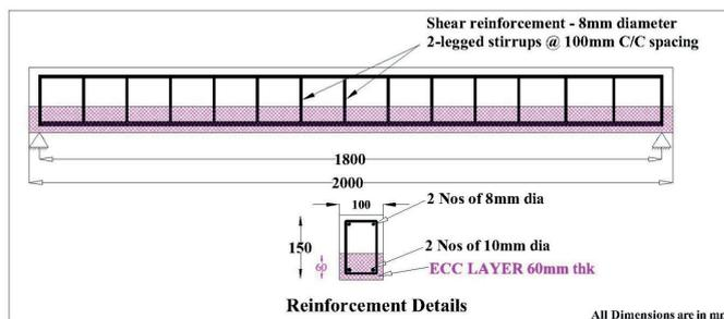
Fig. 4 Dimension parameters, reinforcement details and position of ECC layer
