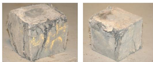
Fig. 7 Typical failure pattern of ECC cubes
