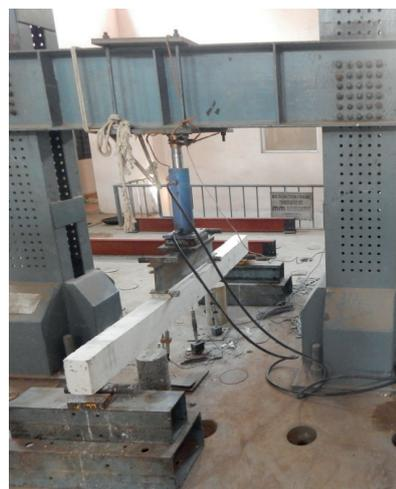
Fig. 5 Four point load test setup on beam
