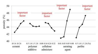
Fig. 3 Impact of the factors level on porosity of hardened mortar Pc (%)
