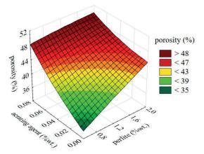
Fig. 6 The impact of perlite (%wt.) and aerating agent sodium C14-16  $\alpha$ -olefin sulfonate (%wt.) on total porosity *Pc* (%)
