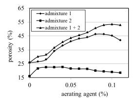
Fig. 10 The impact of the amount of aerating agents: 1 - based on sodium C14-16 α-olefin sulfonate 2 - based on sodium lauryl sulfate (SLS) on porosity Pc (%)
