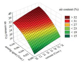
Fig. 4 The impact of aerating agent sodium C14-16 α-olefin sulfonate (%wt.) and cement (%wt.) on air content L (%) in fresh mortars
