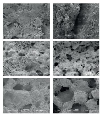
Fig. 9 Photographs of fractures of hardened restoration plaster samples made using SEM, plaster with porosity of 37 % (a and b), plaster with porosity of 42 % (c and d), plaster with porosity of 48%(d and f)
