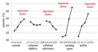
Fig. 2 Impact of the factors level on the air content in fresh mortar L (%)
