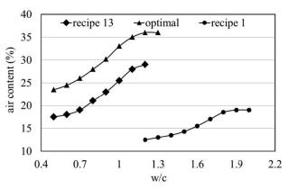
**Fig. 7** The impact of *w/c* on air content in fresh mortars *L* (%) (a), and flow (mm) (b) for samples obtained from recipe 1 and 13 (Table 4) compared with the plasters obtained at the optimal amounts of components (Table 5)
