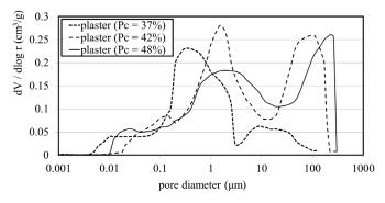
**Fig. 8** Differential distribution of pore volume depending on their effective radii for samples of plasters obtained from recipes 1 and 13 (Table 4) compared with plasters obtained at the optimal amount of components (Table 5)
