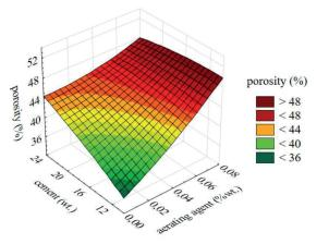
Fig. 5 The impact of aerating agent sodium C14-16  $\alpha$ -olefin sulfonate (%wt.) and cement (%wt.) on the porosity P (%) of renovation plasters
