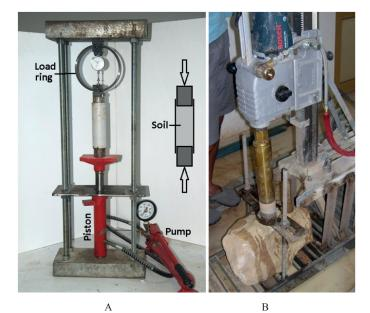
Fig. 3 Sample preparation, A) Static compaction, B) Soft rock coring
