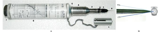
Fig. 1 A) Maruto SH-70 Needle Penetrometer; 1) presser, 2) chuck, 3) penetration scale, 4) load scale, 5) load indicating ring, 6) correlation diagram, 7) removable cap, and 8) penetration needle (Maruto 2006), B) Close up view of the needle
