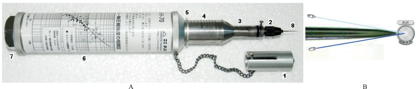
Fig. 1 A) Maruto SH-70 Needle Penetrometer; 1) presser, 2) chuck, 3) penetration scale, 4) load scale, 5) load indicating ring, 6) correlation diagram, 7) removable cap, and 8) penetration needle (Maruto 2006), B) Close up view of the needle
