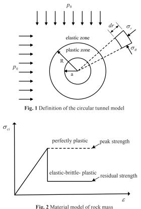
Fig. 2 Material model of rock mass
