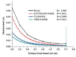
Fig. 10 Displacement comparison of tunnel with rockbolts in numerical analysis
