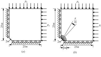
Fig. 9 Numerical model of tunnel
