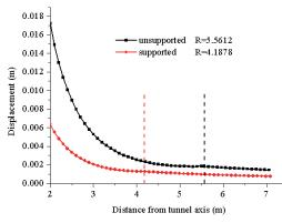
Fig. 7 Displacement comparison of tunnel with or without rockbolts
