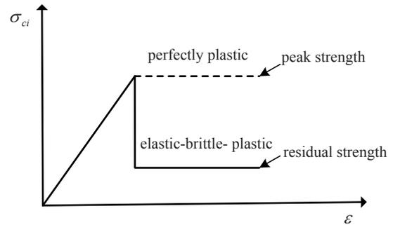
Fig. 2 Material model of rock mass
