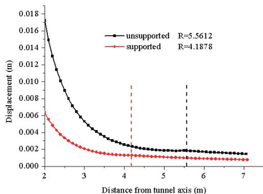
**Fig. 7** Displacement comparison of tunnel with or without rockbolts
