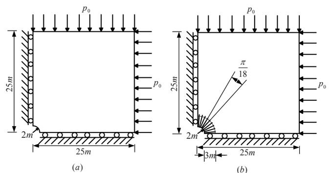
**Fig. 9** Numerical model of tunnel
