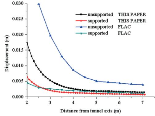
Fig. 11 Displacement comparison of tunnel with or without rockbolts in numerical analysis
