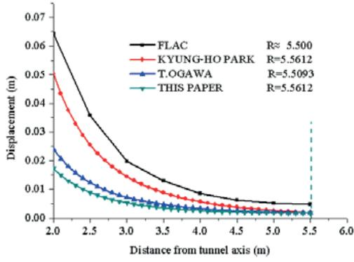
Fig. 10 Displacement comparison of tunnel with rockbolts in numerical analysis
