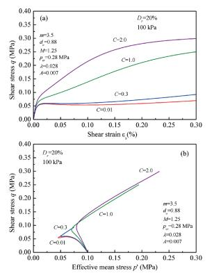
**Fig. 9** Influence of parameter *C* on the computed undrained shear strength and behaviour of granular soils
