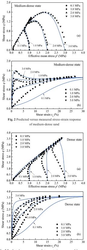
Fig. 3 Predicted versus measured stress-strain response of dense sand
