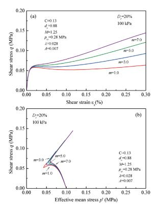
Fig. 8 Influence of parameter *m* on the computed undrained shear strength and behaviour of granular soils
