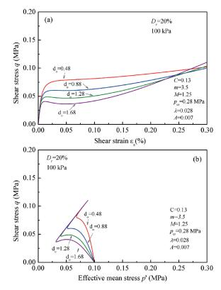
Fig. 7 Influence of parameter  $d_o$  on the computed undrained shear strength and behaviour of granular soils
