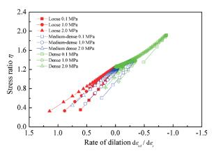
Fig. 5 Stress-dilatancy relationship of sand at different confining pressures and densities
