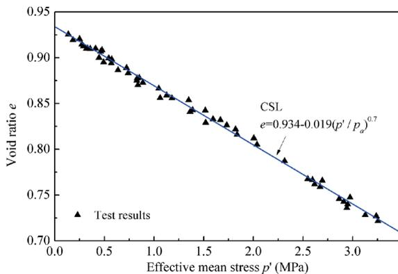
Fig. 6 Determination of the critical state line of sand
