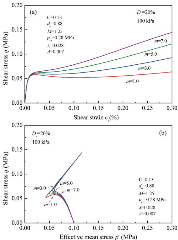
**Fig. 8** Influence of parameter  $m$  on the computed undrained shear strength and behaviour of granular soils
