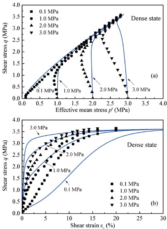
Fig. 3 Predicted versus measured stress-strain response of dense sand
