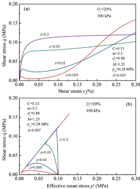
Fig. 11 Influence of compressibility parameter  $\lambda$  on the computed undrained shear strength and behaviour of granular soils
