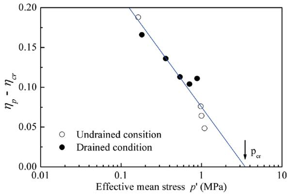
Fig. 4 Determination of the mean stress at the critical state  $p_{cr}$
