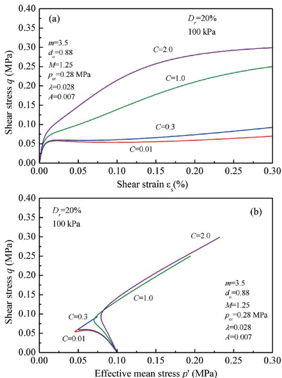
**Fig. 9** Influence of parameter  $C$  on the computed undrained shear strength and behaviour of granular soils
