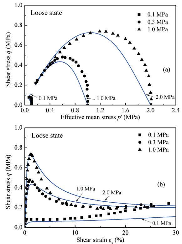
Fig. 1 Predicted versus measured stress-strain response of loose sand
