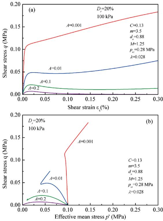
Fig. 10 Influence of shear deformability parameter  $A$  on the computed undrained shear strength and behaviour of granular soils
