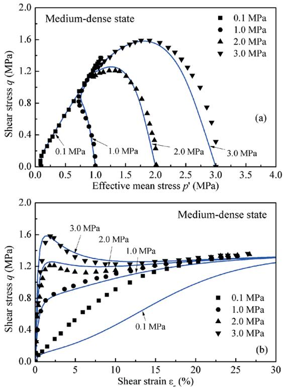
Fig. 2 Predicted versus measured stress-strain response of medium-dense sand
