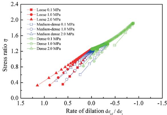
Fig. 5 Stress-dilatancy relationship of sand at different confining pressures and densities
