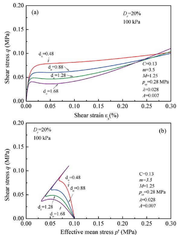
Fig. 7 Influence of parameter  $d_o$  on the computed undrained shear strength and behaviour of granular soils
