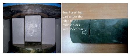
Fig. 8 a) Specimen loading, b) a failed specimen with minor crushing (spalling) under  $15^{\circ}$  jaw and a = 3mm condition
