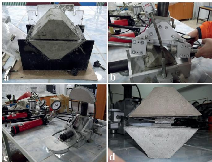
Fig. 1 a) Moulding in conventional shear strength test, b and c) Loading equipment, d) a failed specimen
