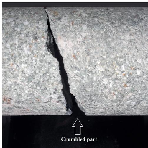
**Fig. 6** Failure under the loading condition of  $a = 0 \text{ mm}$  and  $b = 60 \text{ mm}$  ( $\alpha = 180^\circ$ )
