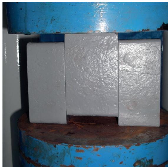
Fig. 3 Double shear jaw under loading
