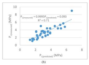
$\textbf{Fig. 17} \ Correlation \ of \ a) \ P_{_L} \ and \ w\% \ and \ b) \ P_{_{L \ (measured)}} \ and \ P_{_{L \ (Predicted)}} \ with \ three \ variables \ in \ clayey \ soils$
