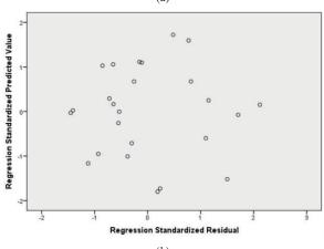
$\label{eq:Fig.4} \textbf{Fig. 4} \text{ a) correlation of } E_{_{M}} \text{ and } N_{_{60}} \text{ values in sandy soils, b) } \text{Residual analysis} \\ \text{result for } E_{_{M}}\text{--}N_{_{60}} \text{ relationship}$
