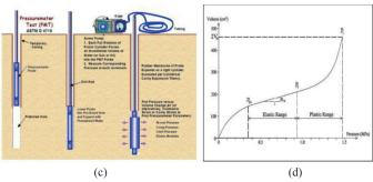
Fig. 1 Diagrams depicting the principles of the (a) SPT test, (b) UCS test, (c) Pressuremeter test and (d) a typical pressuremeter graph.
