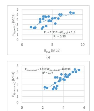
**Fig. 9** Correlation of a)  $P_L$  and  $E_{UCS}$  and b)  $P_{L \text{ (measured)}}$  and  $P_{L \text{ (Predicted)}}$  with two variables in sandy soils
