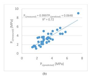
$\textbf{Fig. 19} \ \text{Correlation of a)} \ P_{L} \ \text{and PI\% and b)} \ P_{L(measured)} \ \text{and} \ P_{L(Predicted)} \ \text{with four variables in clayey soils}$
