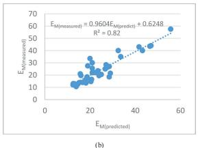
$\label{eq:energy} \textbf{Fig. 14} \ Correlation \ of \ a) \ E_{_M} \ and \ E_{_{UCS}} \ and \ b) \ E_{_{M(measured)}} \ and \ E_{_{M(Predicted)}} \ with \ two \\ variables \ in \ clayey \ soils$
