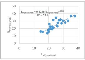
$\label{eq:Fig. 8} \textbf{Eorrelation of a)} \ E_{\text{M}} \ \text{and} \ E_{\text{UCS}} \ \text{and b)} \ E_{\text{M(measured)}} \ \text{and} \ E_{\text{M(Predicted)}} \ \text{with two}$  variables in sandy soils
