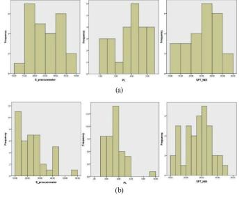
Fig. 3 Histograms of the in situ test data (a) sandy soil and (b) clayey soil (pressuremeter modulus  $(E_M)$ , limit pressure  $(P_L)$  and corrected SPT blow count  $(N_{co})$ )
