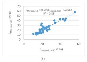
$\textbf{Fig. 18} \ \ Correlation \ of a) \ E_{M} \ and \ PI\% \ and \ b) \ E_{M(measured)} \ and \ EM(Predicted) \ with \ four \ variables \ in \ clayey \ soils$
