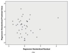
Fig. 13 a) correlation of  $P_L$  and  $N_{60}$  values in clayey soils, b) Residual analysis result for  $P_L$  -  $N_{60}$  relationship
