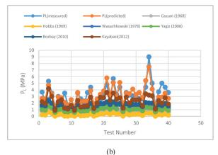
**Fig. 11** Comparison of the measured and estimated values of a)  $E_M$  and b)  $P_L$ , estimated from other empirical equations for clayey soils
