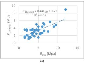
$\textbf{Fig. 15} \ Correlation \ of \ a) \ P_{L} \ and \ E_{UCS} \ and \ b) \ P_{L \ (measured)} \ and \ P_{L \ (Predicted)} \ with \ two \ variables \ in \ clayey \ soils$
