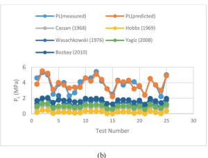
$\label{eq:Fig. 6} \textbf{ Comparison of the measured and estimated values of a) } E_{\rm M} \ \text{and b) } P_{\rm L},$  estimated from other empirical equations for sandy soils
