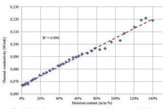
Fig. 6 Relation between moisture content and thermal conductivity
