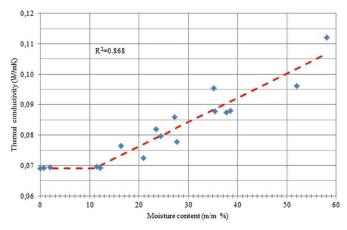
Fig. 1 Relation between moisture content and thermal conductivity in Experiment 1 [10][11]
