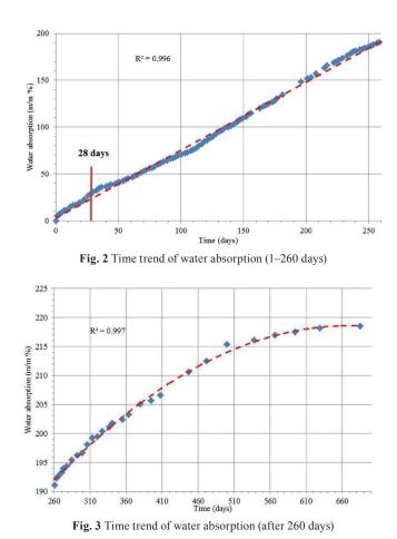
It was also found that water absorption of nano-ceramic coating is 6% in the first 24 hours. Examining the further development of water absorption it can be concluded that after the first day evolution of water absorption continues along a linear function (Fig. 2).
