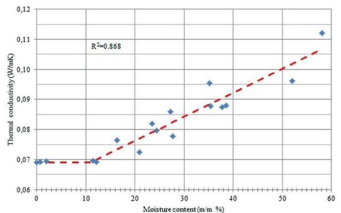
Fig. 1 Relation between moisture content and thermal conductivity in Experiment 1 [10][11]
