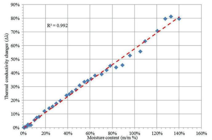
Fig. 7 Relation between moisture content and thermal conductivity changes
