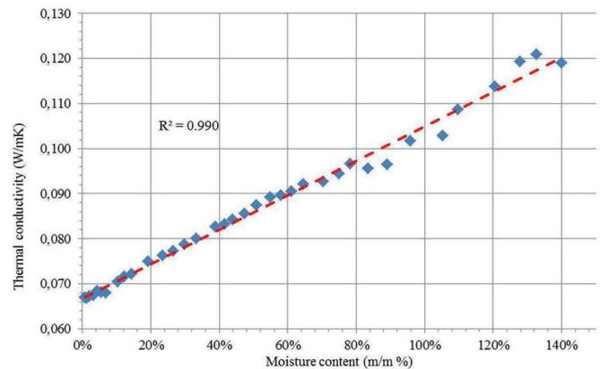
Fig. 6 Relation between moisture content and thermal conductivity
