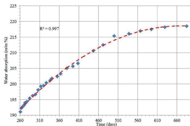
Fig. 3 Time trend of water absorption (after 260 days)
