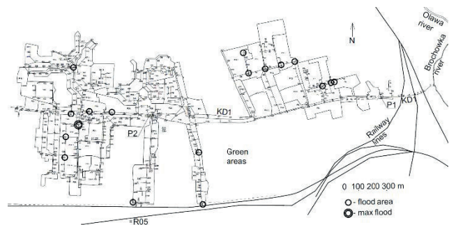
Fig. 5 Localization of floodings from stormwater drainage system for actual rainfall with C = 5 years and t = 42 minutes
